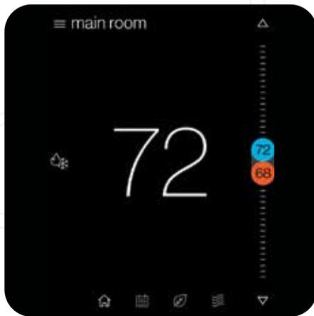
The **home screen** displays the current temperature, the current system mode, and adjustment slider, as well as icons leading to the top level screens.
