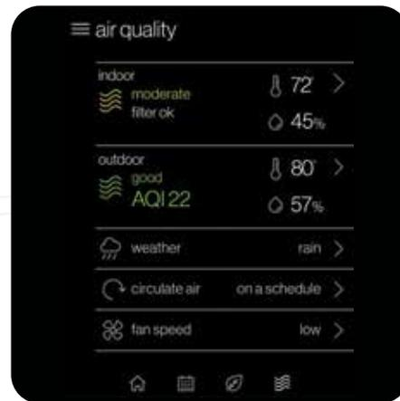
The **air quality screen\*** displays indoor air quality levels when a Daikin *One* home air monitor is connected. Outdoor air quality and weather will be displayed when connected to the internet and thermostat added in the mobile app under home location.
