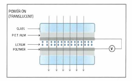
When the electrical supply is removed and the power is switched **off**; these liquid crystal molecules relax into a random orientation. This diffuses and scatters the light that is transmitted through the glass and the Privacy Smartglass appears opaque (private).
